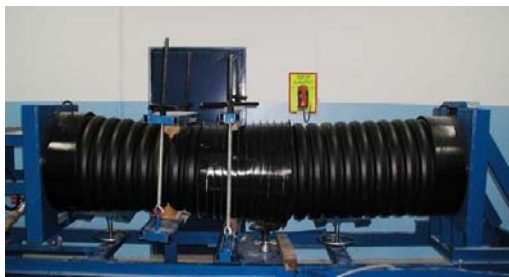
Leak tightness test
