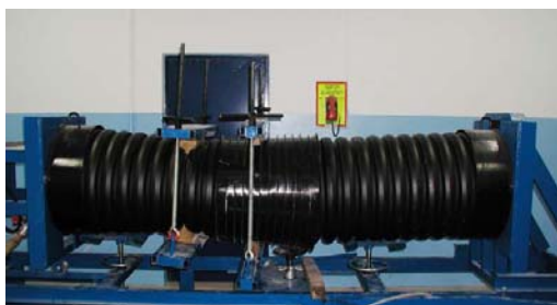
Leak tightness test
